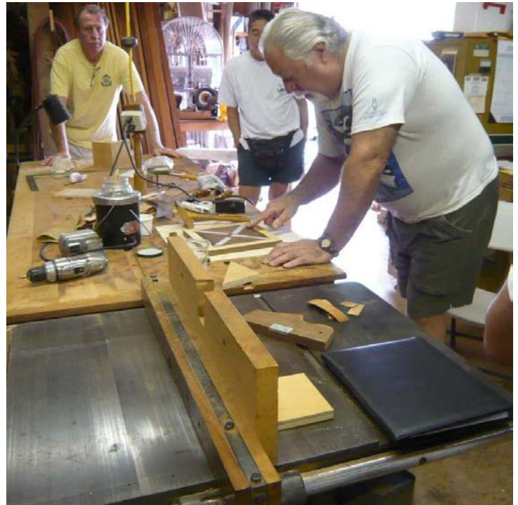
Alfred Sharp demonstrates hammering veneer using hot hide glue at Alan Wilkinson's workshop in Honolulu. Photos by Rosalind Young.
