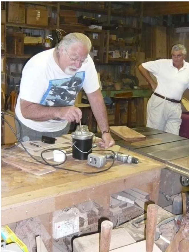
Alfred Sharp demonstrates hammering veneer using hot hide glue at Alan Wilkinson's workshop in Honolulu. Photos by Rosalind Young.
